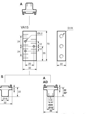
\* Dimension on A-end at AD actuation
