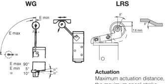
Maximum actuation distance, the maximum spool stroke length is 7.6 mm. ۲
